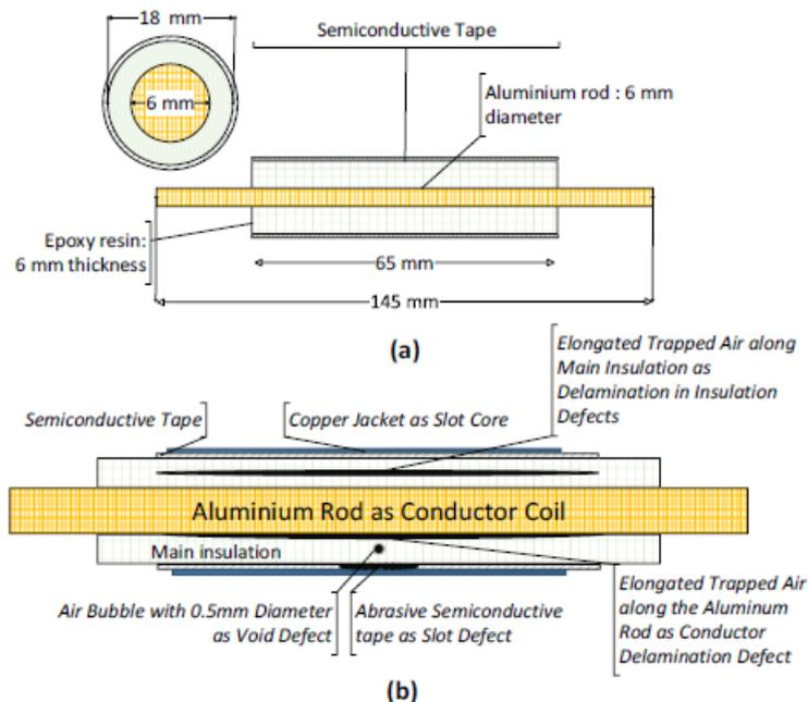
**Fig. 2.** (a) Simplified physical design of a rotating machine insulation model, and (b) representation of various defect types simulated in the model (actually, each model only has one defect type)
