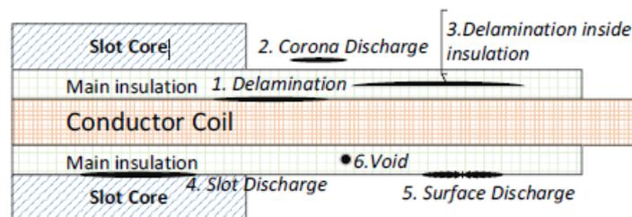
**Fig. 1.** Common PD-related defects in a rotating machine insulation
